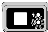
Autofocus lamp blinks slowly to show that pictures can not be accurately framed in viewfinder
